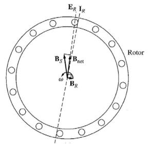
On the left is a figure of the magnetic fields in an induction motor at no load
