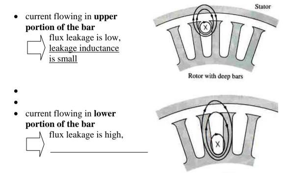
Since all parts of the rotor bar are parallel electrically, the bar essentially represents
