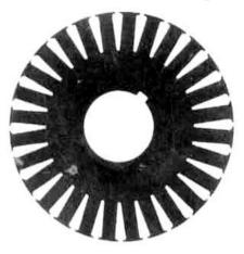
**Upper part** of a deep rotor bar: the current flowing is tightly coupled to the stator, and hence the **leakage inductance is small** in this region.
