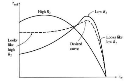
Torque-speed characteristics curve combining highresistance effects at low speeds (high slip) with low resistance effects at high speed (low slip).
