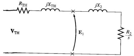
**Source impedance** =  $Z_{\text{source}} = R_{\text{TH}} + jX_{\text{TH}} + jX_2$
